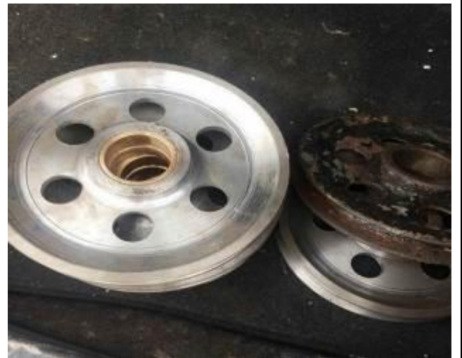
New fabrication of sheave
