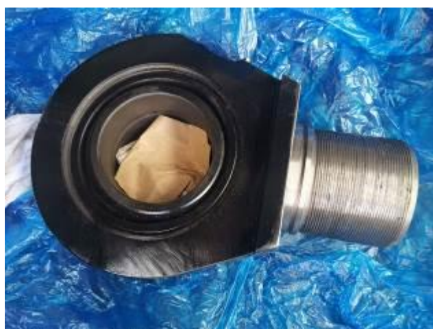
New fabrication of hydraulic ram knuckle
