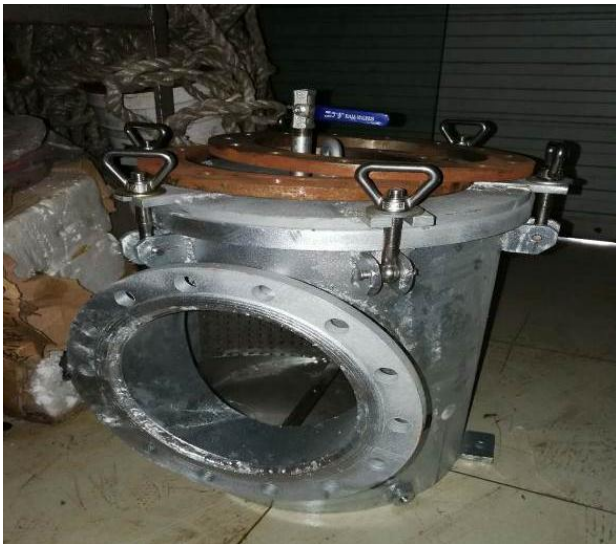
New fabrication of sea water strainer
