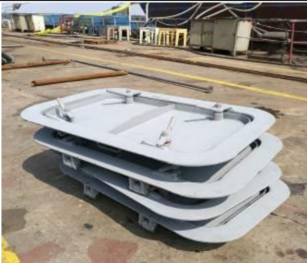
New fabrication of water-tight door
