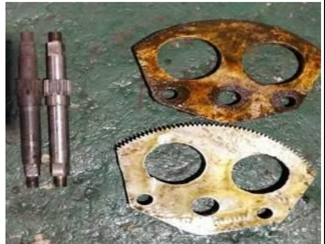
Special gear for water-tight door
