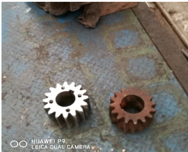
New fabrication of gear
