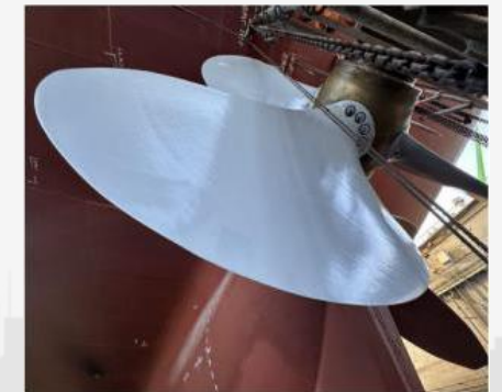
XGIT-Prop coating system: provides a smooth, low-energy finish to avoid biofouling to adhere to the surface
