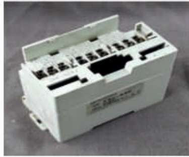
MITSUBISHI FX2N 4AD PROGRAMMABLE CONTROLLER
