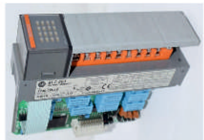
ALLEN BRADLEY OUTPUT MODULE
