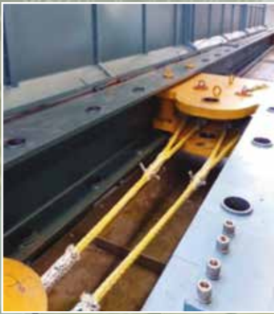
Angled Endurance testing for mooring lines according to MEG4 specifications.
