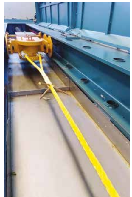
Axial Compression resistance testing for mooring lines according to MEG4.
