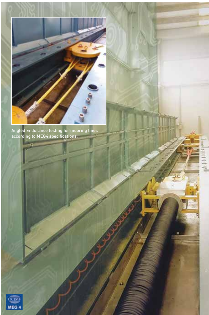
Testing for Line Design Break Force, as per MEG4. Evaluating your mooring line's strength.
