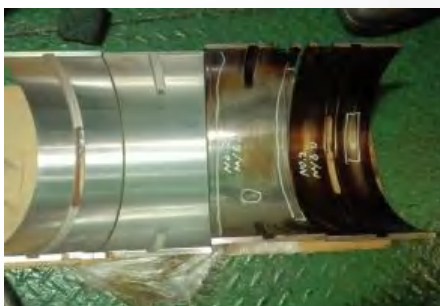
A/E&M/E Bearing Inspection
