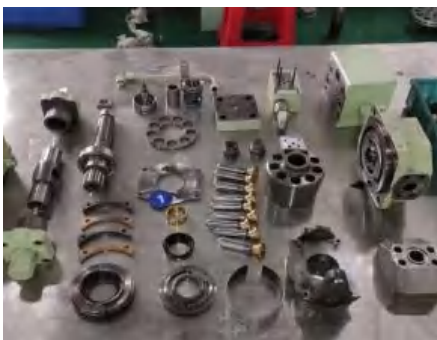
HPS Pump Overhaul
