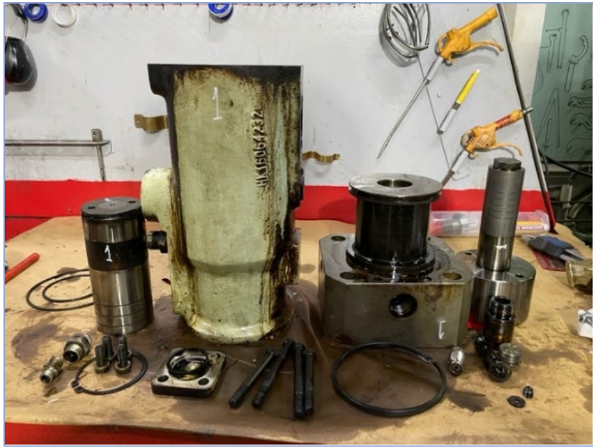
Hydr. booster and pump unit, inspection/ measuring of pistons/sleeves and suction valves.
