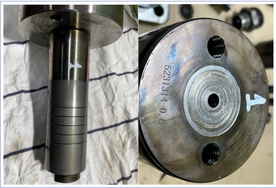
Piston and surfaces of booster with exceed wear.
