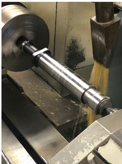
Fuel pump barrel and plunger reconditioning
