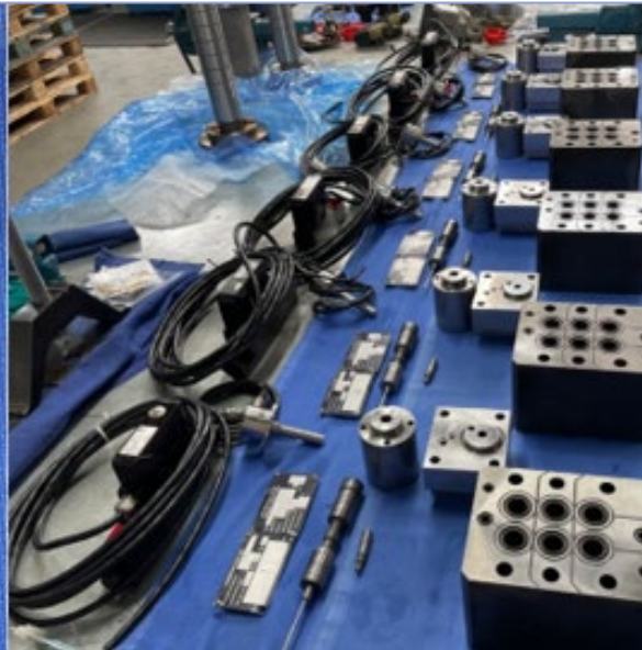
ELFI control valve incl. proportional valve and feedback sensor.
