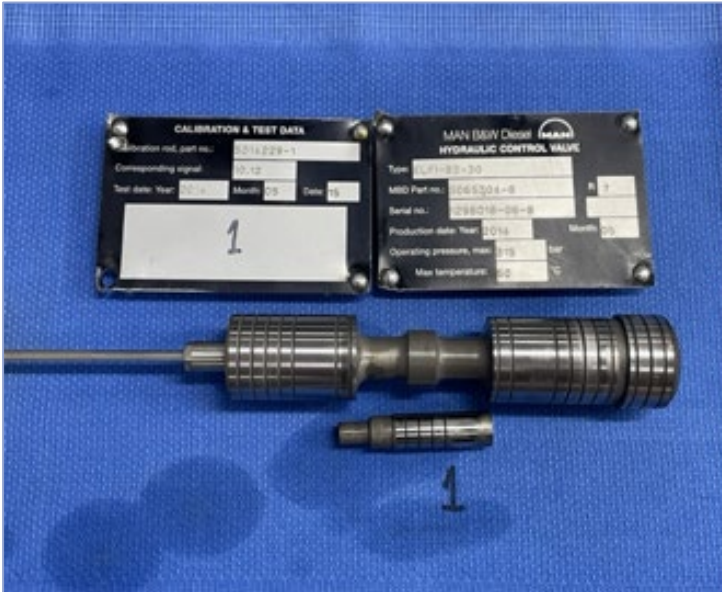
ELFI control valve incl. proportional valve and feedback sensor.
