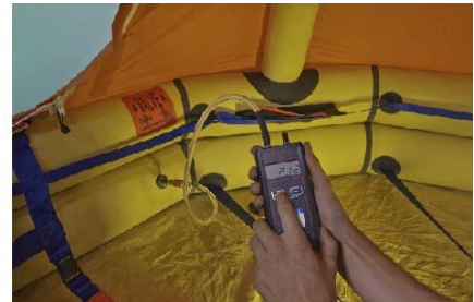
WORKING PRESSURE TESTING
