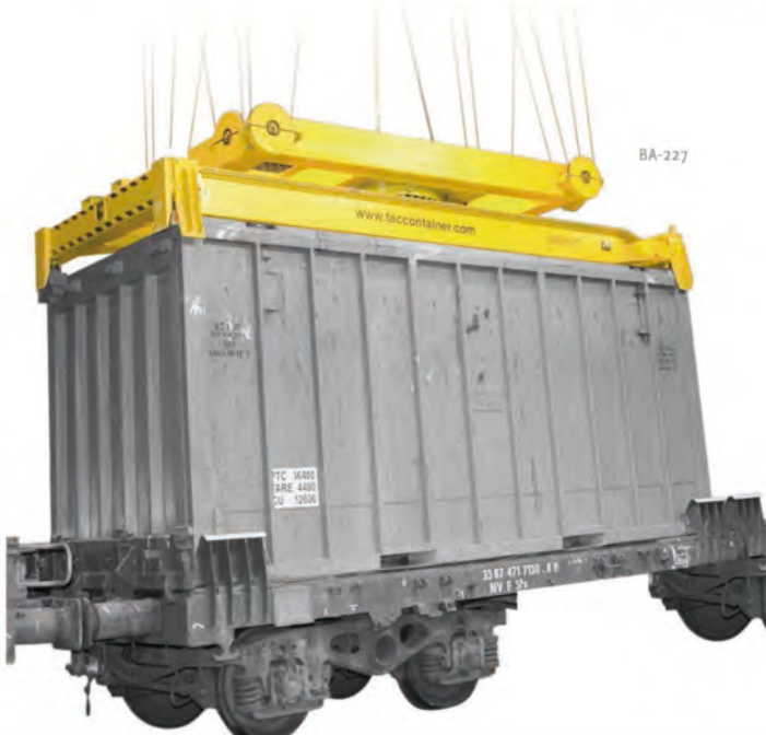
Telescopic 20'-40' spreader with flippers and gravity point regulator
