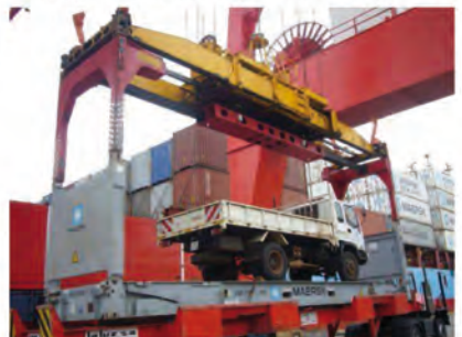
BA-030ET telescopic 20' to 40', TTI terminal Algeciras
