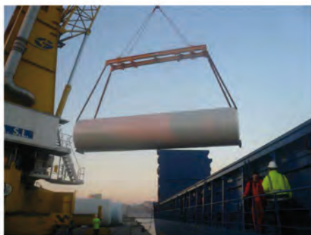
Frame BA-190 loading wind tower section
