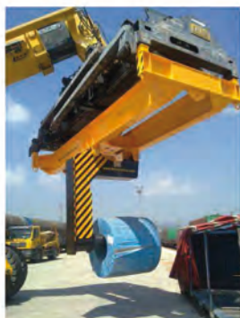
BA-110P handling coil in ADIF facilities
