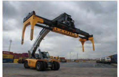
BA-030ET telescopic 20' to 40', ADIF train terminal
