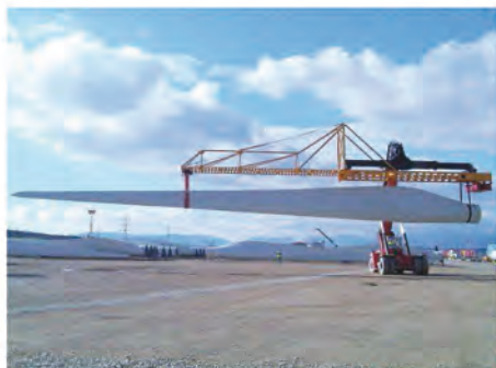
Prototype BA-249 testing in Gamesa facilities
