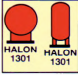
6669 Halon 1301 bottles placed in protected area
