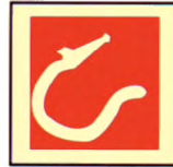
6683 Hose box with spray/jet fire nozzle
