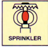
6658 Space protected by sprinkler
