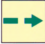
6704 Secondary means of escape
