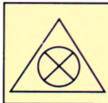
6726 Remote ventilation shutoff
