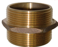
358-2525-57 Double Male 2-1/2" NST Adapter for Joining Two Tank Cleaning Hose Couplings. Brass.
