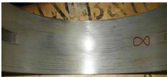
Bearings after a running time of 15,000 hours
