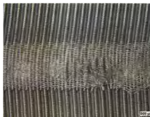
Low cost supplier: Weld seam
