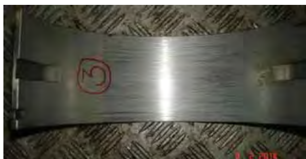
Bearings after a running time of 15,000 hours
