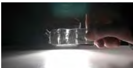
Filter fabric 10µm ( mesh 660/63 ) before cleaning
