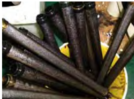
Candle filter before cleaning in ultrasonic bath
