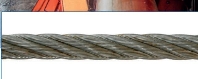
Standard wire rope with higher breaking strength. Used for all kinds of purposes, i.e. luffing, mooring, towing, anchoring and coupling push barges. The independent wire rope core provides more strength and stability to the wire rope compared to a fibre core. Construction is according to ISO standard.
