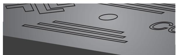
Easy wear detection by prefabricated grooves of 1mm, 2mm and 3mm deep. Based on positions where pads wear down most.
