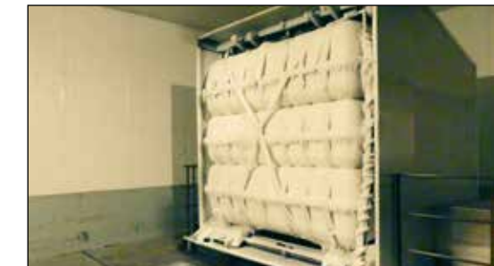
VEC Plus™ ice tested at -30°C with 60 mm ice cover
