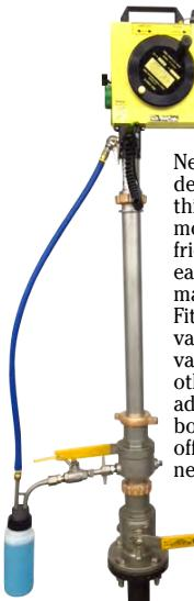
New modular design makes this sampler more user-friendly and easier to maintain. Fits most MMC vapor control valves; fits others with adaptor. Sample bottle twists off quickly and neatly.
