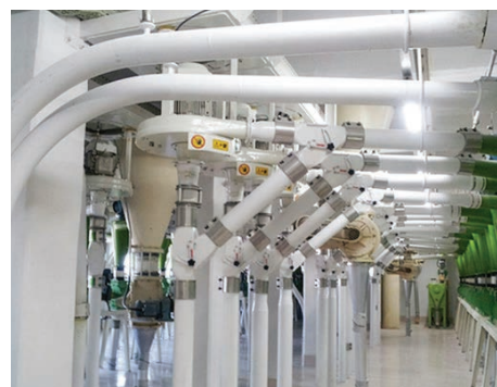
MJS EPDM + strip insert 80A~125A. wheat flour conveying system. Korea
