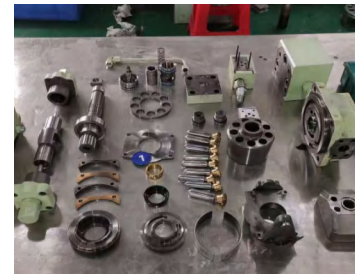
HPS Pump Overhaul
