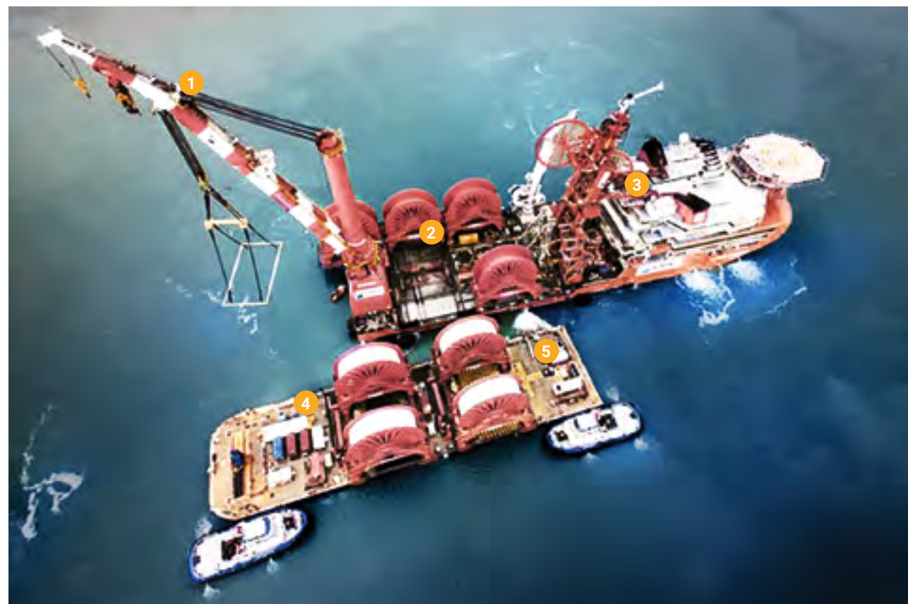
1 Controlling Load Moments 2 Combined Blower Heel Control and Roll Damping system 3 Loading Computer with Crane Operation Simulation 4 Heel Control system with Zero-Flow 5 Draft Measurement, Tank Content Measurement and Valve Remote Control system
