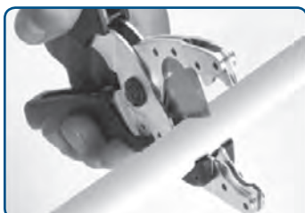
1. Cutting the pipe.
