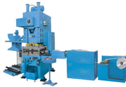
HEAT EXCHANGER COOLER FIN PRESS MACHINE
