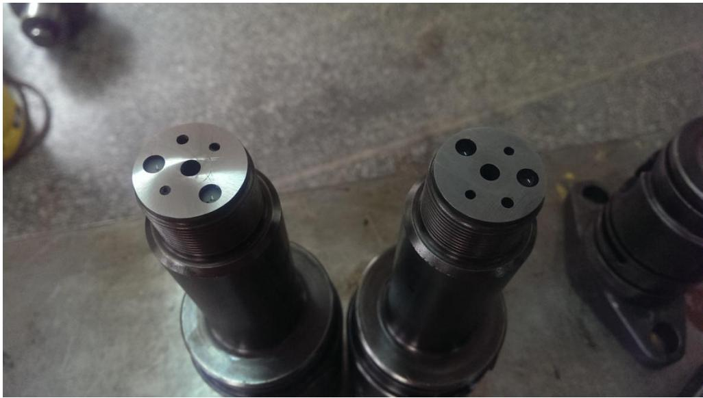
The fuel injectors with damaged surface or wear in the middle of the surface create the problems below:
